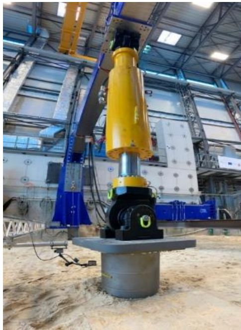
FIGURE 4.5 SCALED UMACK TEST ANCHOR UNDER LOAD TEST AT IWES FACILITY.
