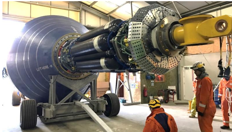
FIGURE 4.3 CORPOWER C 4 WEC
